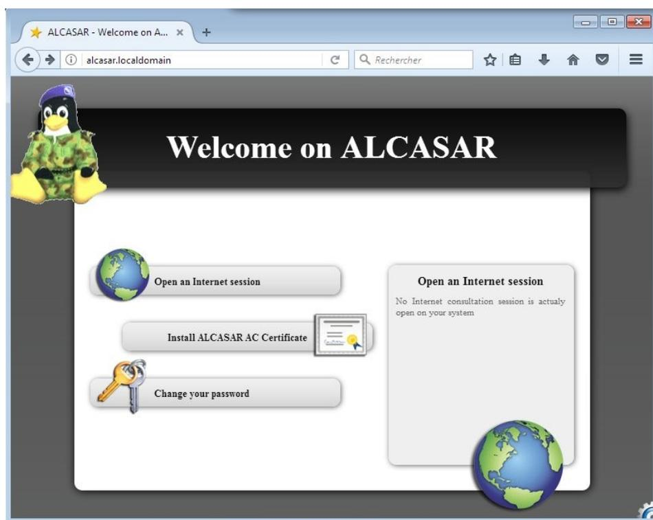
Click on the small crated wheel at the bottom right in order to connect to the ALCASAR Control Center (ACC). You must authenticate you with the first account created during the installation process (§2.3 – P10 of this document).
